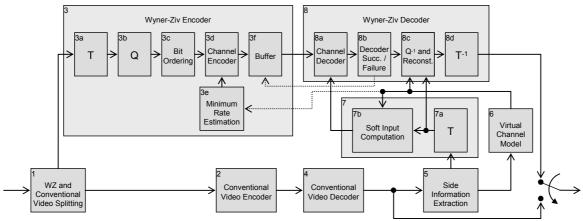
Figure 1. Block diagram of the DISCOVER architecture. Dotted lines represent the feedback channel.
