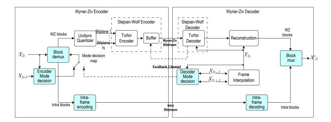
Fig. 1. IST-PDWZ video codec architecture
